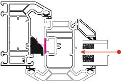
It may be necessary to pack the sash/glass at this point as shown
