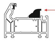
Fit a 17mm Frame Wedge to the outer frame on the stay fixing area
