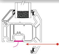
Fit a Sash Spring to the sash on the center line of the stay fixing area
